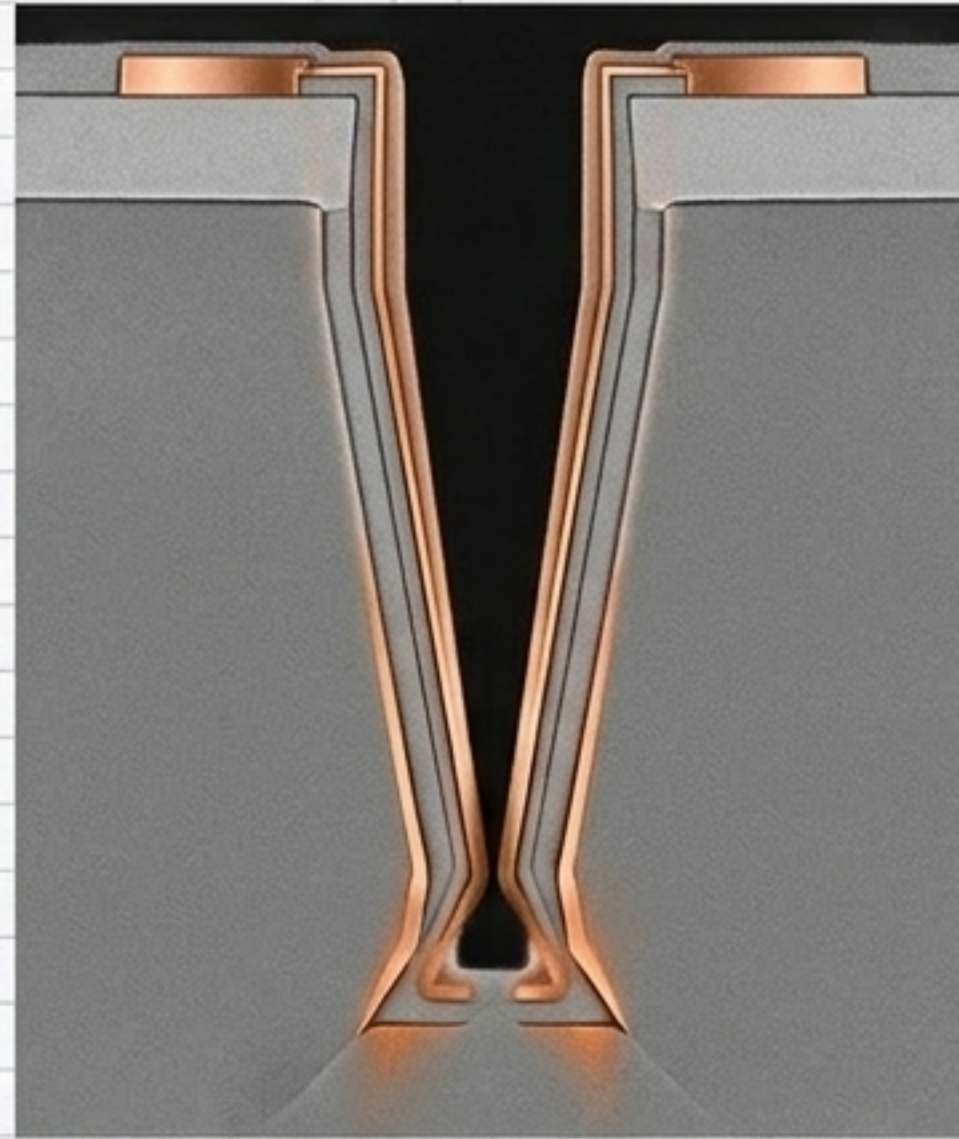
Yield Failure (Tapering / Cannot hold charge)
